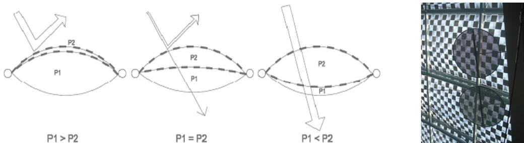
Fig. 4. (a) active shading strategies. Source: Own elaboration; (b) active shading inflatable envelope in Esslingen, by Form-TL. Source: Own photo
